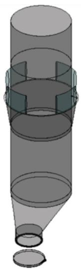
XELTA Pac has a bigger diameter at the top opening, which enables easy filling, accurate weight adjustment and easier product discharge. This design has a large fill neck, allowing easier charging/dispensing into the bag. This reduces fill time and lowers the risk of spillage when filling the bag.
