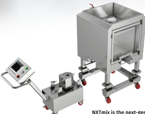
NXTmix is the next-generation levitation-based mixing technology designed to handle all your single-use mixing requirements from media & buffer preparation, intermediate process mixing, final formulation and filling application. Highly flexible and cGMP complaint system allows you to use volumes commonly used in manufacturing processes of up to 1000L.
